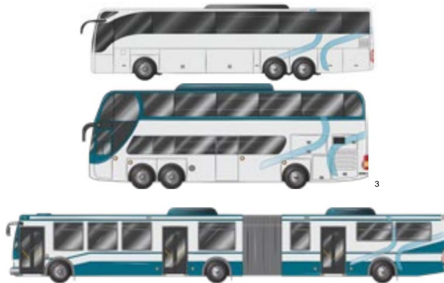
Figure 1. Three-axle bus variations: three-axle bus or coach; three-axle double decker; three-axle articulated bus
